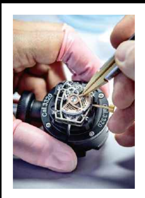
The variable-geometry rotor in gem-set red gold is gently set in place
