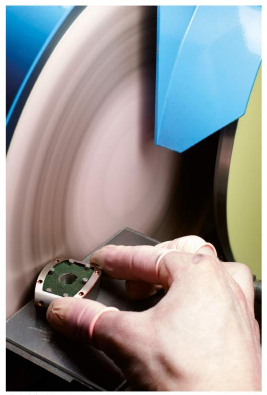
Hand polishing of the outer bezel edges of an RM 07-01 ladies watch. This provides an elegant counterpoint to the brushed upper surface of the bezel, visible here.
